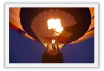
A hot air balloon has three major parts: the basket, the burner, and the envelope. The basket is where passengers ride. The basket is usually made of wicker. This ensures that it will be comfortable and add little extra weight. The burner is positioned above the passenger's heads and produces a huge flame to heat the air inside the envelope. The envelope is the colorful fabric balloon that holds the hot air. When the air inside the envelope is heated, the balloon rises.
