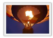
A hot air balloon has three major parts: the basket, the burner, and the envelope. The basket is where passengers ride. The basket is usually made of wicker. This ensures that it will be comfortable and add little extra weight. The burner is positioned above the passenger's heads and produces a huge flame to heat the air inside the envelope. The envelope is the colorful fabric balloon that holds the hot air. When the air inside the envelope is heated, the balloon rises.
